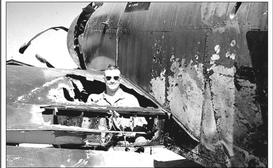
Capt Russ Everts stands in the monzombus hole in the left wingroot area caused by an in-flight fire due to battle damage. The Skyraider most likely was working Steel Tiger and was in need of a foamed runway which would not have been available at Pak Se, which would have been the closest suitable landing field from the Bolovens Plateau area of Southern Laos. The question was posed...who flew this mission?...and Jon Ewing answered the mail. Courtesy of Skyraider.org
